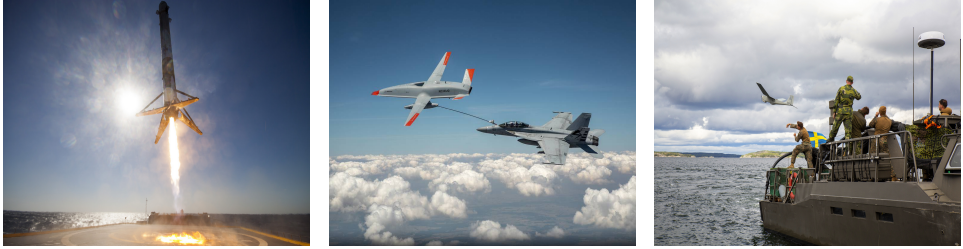
Figure 1.1: Examples of cooperative multi-domain operations with manned or unmanned agents. SpaceX rocket landing on the autonomous drone ship (USV), Boeing UAV conducting aerial refueling of an aircraft, Swedish and US marines using a UAV and ship radars for surveillance. Image credit: SpaceX/Boeing/DoD
